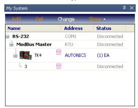
Selecting the unit address (3) enables Change button. To change the unit address, click the Change button on the tab or right-click on mouse to select Change.
