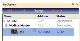
Selecting TK4 device enables Add button. To add a unit(address), click the Add button on the tab or right-click on mouse to select Add.
