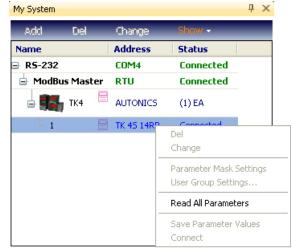
When the reading is completed, the Property window displays the parameters. Parameter change is also available.
