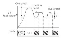
As like above picture, the control value is up and down by set value, it is called Hunting. And Overshoot is occurred at initial point when just nower on
