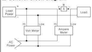
\*When measure over DC2A, please use Shunt and measure over AC5A, please use C.T. (Current Transformer).
