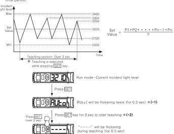
•In case incident light level is received under 10DIGIT while teaching, [Errt] will be flickering twice and return to RUN mode with previous SV retained.
