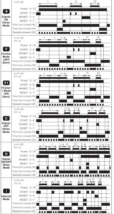
Note) 1. If the power supply is off or the terminals ② and ⑦ are shot-circuited (RESET signal is ON) the time progressing will be reset.
