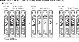
①Channel No. is indicated on PV display part and [et] is indicated on SV display part for master unit while COPY is executed.
